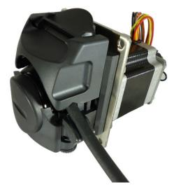
Generally, stepper motor driven pumps work best in very low flow applications. For this reason, the flow rates in the chart below are given in milliliters per revolution. The motor controller, tubing type and size, fluid viscosity, number of rollers, and back pressure will determine actual flow rate, psi and current consumption.
